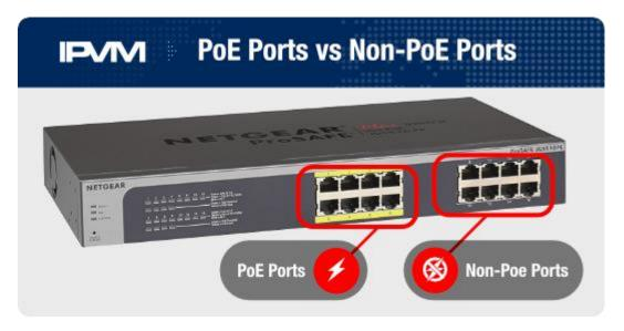
These switches can have all or only some ports PoE capable (with the others being data only ports).
