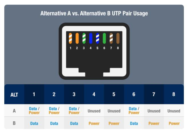
Most surveillance devices today will auto sense which pairs are used for data and power, meaning that most devices are Alternate A or B agnostic.
