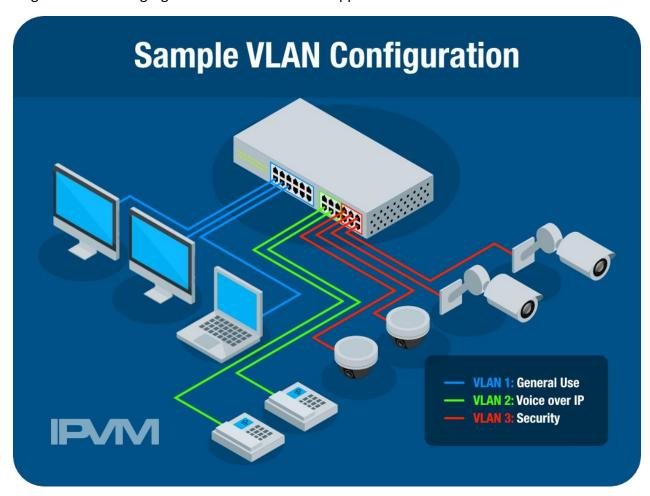
VLANs can be static or dynamic. In a static VLAN, the switch port that the device is connected to determines the VLAN ID.
