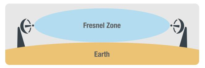
Wireless links are sensitive to environmental factors and fluctuations in site conditions, making maintenance a key consideration when deploying wireless. Things such as antenna alignment, corrosion on the connectors, foliage in line of sight, etc. should be checked periodically.
