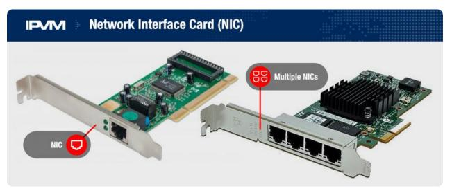
This image shows what a multi-NIC dedicated card looks like. It is possible for a computer to have multiple NIC's in a mixed wired and wireless network, where the wired port is one NIC and the wireless function is separate NIC.
