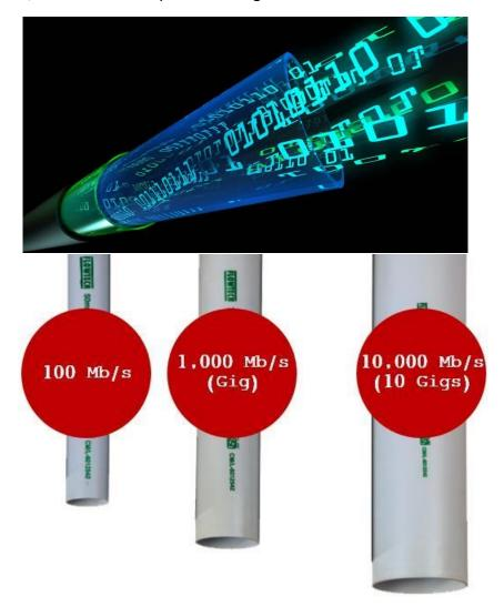
Higher speed capacities do not necessarily mean a physically bigger cable or medium. For example, Cat5e can handle up to 1 Gb/s. Cat6 can handle up to 10 Gb/s. Single mode fiber can handle up to 40 Gb/s, therefore is the biggest 'pipe' while being physically the smallest of the three examples.
